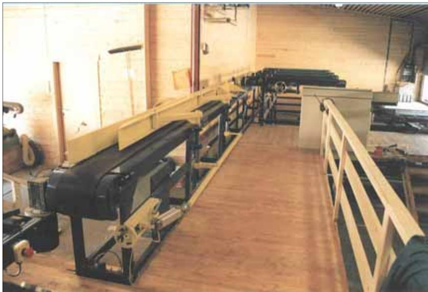
A heavy duty belt conveyor equipped with a moving guide mechanism designed to keep the timber upright until it has entered the strength testing machine. On entry to the machine the guide will automatically be removed to prevent interference with the grading process.
