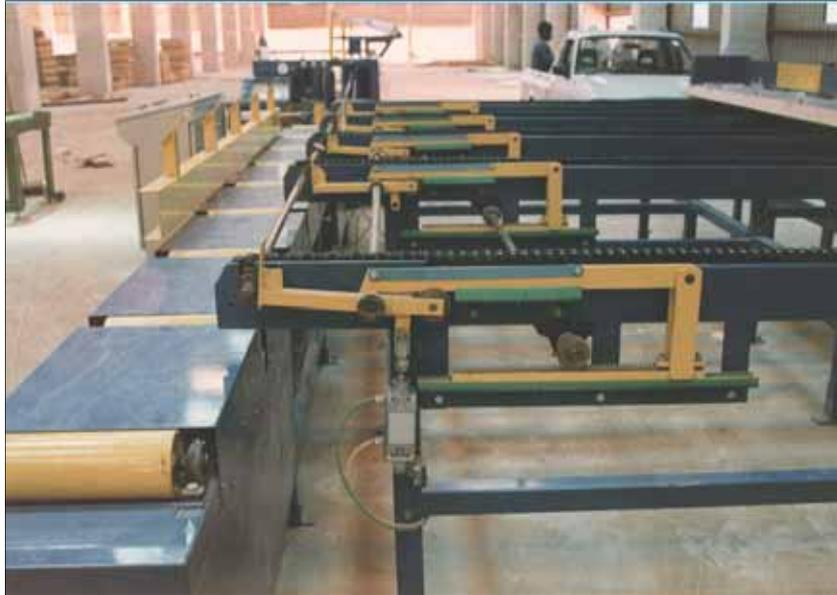
This apparatus is a four or five strand chain which employs a width adjustable hold and release mechanism, designed to hold back all timber allowing only the first piece to be released to the infeed conveyor. The profile of the feeder together with the infeed guide are responsible for turning the timber on edge ready for grading.
