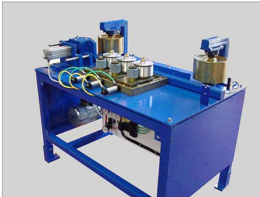
This marker is a self powered marker which employs pneumatically operated ink rollers to effect a grade mark down the full length of the timber. The marker is produced to give a maximum of four grade marks but is also available in two and three marker arrangements. Inking is by exchange pre-inked roller pads of either soakable or dispensable types.
